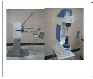
The strength of materials lab is to demonstrate the principles of the mechanics of materials and structural analysis to the students through a series of experiments. In this lab, the experiments are performed to measure the properties of the materials such as tensile strength, impact strength, compressive strength, hardness, etc.
